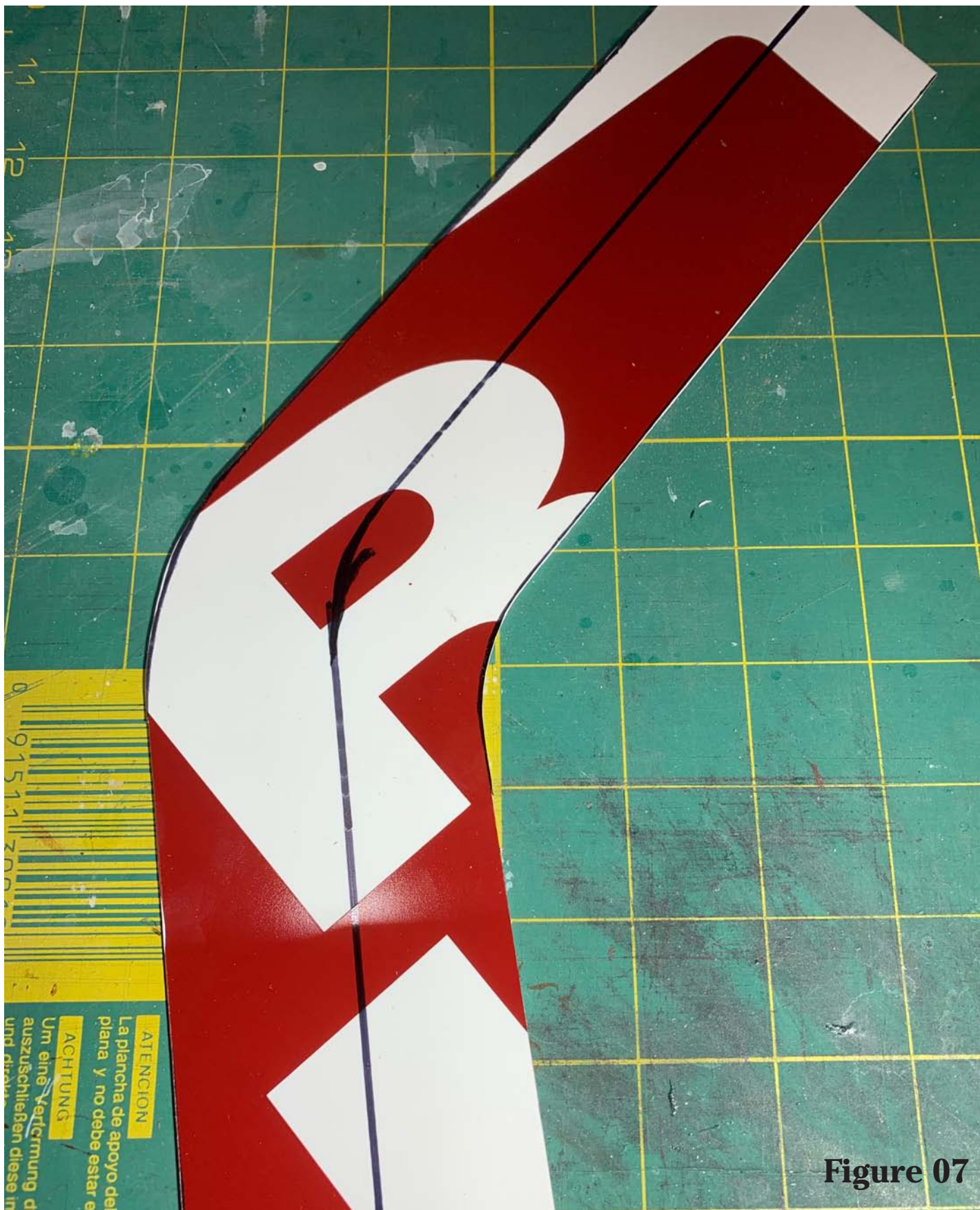
Figure 07 I cut the foam board along the edges of the stencil with a sharp hobby knife. I try to get all the way through the foam core in one pass to avoid jagged edges. I position the same stencil over the plastic sign and scribe along the edges of the stencil with the sharp hobby knife. For the plastic, the knife doesn't cut all the way through. It's enough just to make a shallow groove. If you bend the plastic, it will snap cleanly along the groove.
