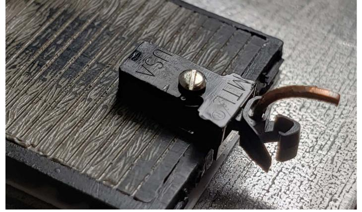
Fig 11. Lightly sand off the details on the former deck, now the underside of the car. Then mount MT 1023 couplers using a 00-90 screw that will go through the body but not hit the underside of the new deck. Nominally the screw can penetrate 3/32" into the car without touching the deck. The screws should self tap into the plastic.
