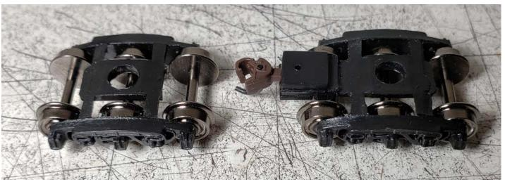
Fig 6. Lets turn our attention to the trucks now. I decided to reuse the Buckeye trucks that came with model. The side frames are a bit thick, however the relief is pretty good. Cut off the truck mounted coupler as shown on the truck on the left.
