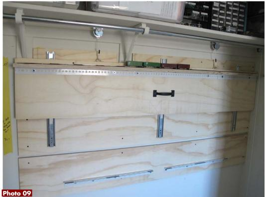
coming from the layout will determine where on the elevator's rise you will need to install a stop. I used a barrel slide bolt at that point. Since all of my traffic comes onto the elevator locomotive first, I made the approaching track coming from the layout with an uphill grade of 1% or so. Thus, when the train had to back out, it would be going slightly downhill, relieving some of the stress on the locomotives and couplers and, hopefully, reducing any derails from the push.
