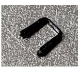
Fig 14. I felt this car needs some detail like stirrups, but how to mount them? I had several leftover MT 3001 stirrups that had one side that had been broken and thus replaced. I found I could cut the remaining stirrup off the cross piece.
