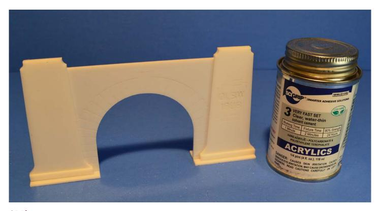
**O5 Above.** Assembly. Once all the parts are manufactured, it's time to assemble the pieces. A thin paper layer that normally protects the sheet from scratches should be peeled off after the cutting process. Acrylics should be bonded with a compatible acrylic cement
