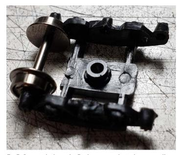
Fig 7. One quirk about the Bachmann trucks is they normally use a body mounted center pin to hold the truck with a screw to retain the truck on the pin. To accommodate this the hole in the truck is rather large. The way to retrofit these to a more conventional mounting method is shove a Micro Trains bolster plug in the hole. These were originally made to plug the large holes in the underframes of ConCor cars so you could use Kadee trucks and bolster pins.
