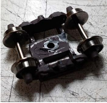
Fig 8. Use a hot solder iron to melt the plug to the truck frame. Then trim the plug protrusion flush with the truck frame. The reason this is important is because the screw used to hold the truck on will interfere with the center axle if the plug is not trimmed.
