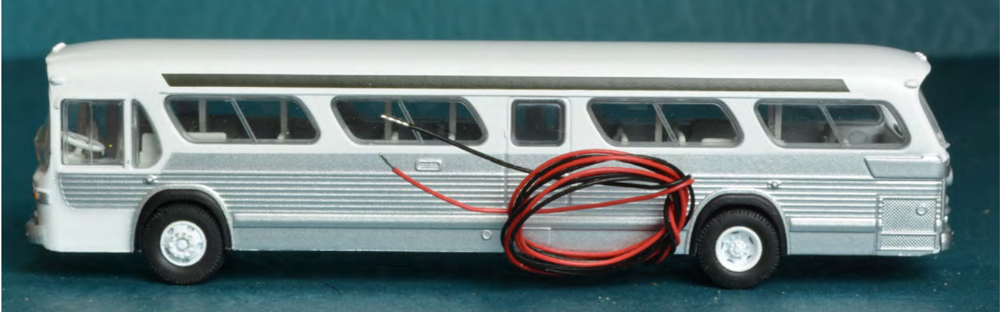
Above. The New Look busses are out! Santa Monica 2525 is Rapido 573008. Below. White/Silver Undec is Rapido 573098. Notice the wires to light the head and tail lights. To be certain to not exceed the 12V DC maximum, Rapido recommends using a 9 volt battery. A great idea!
